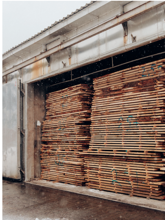
Processed wood in the sawmill's drying chambers
